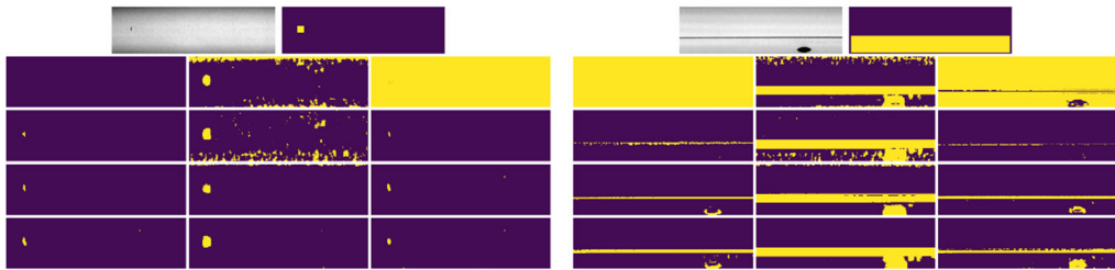
Figure 4. We show a forward pass of a single image of steel producing a dense segmentation over refinement sessions with three different experiments. This is accomplished via the graphical interface where the user is given the 5 worst negatives and positives based on an anchor, then selects new centre pixel for that patch. Row one displays the image and the initial mask. Column one is based on user refinement, column two is mask updates, and column three is user refined with entropy anchor selection. Each row shows a subsequent refinement after a session.
